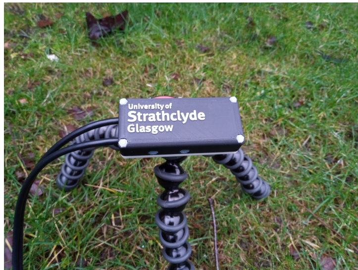
Figure 1. Photograph of the field-deployed DC OPM, which may be operated as a PID-locked double-resonance sensor or a digital self-oscillator, to achieve high dynamic range and bandwidth.
