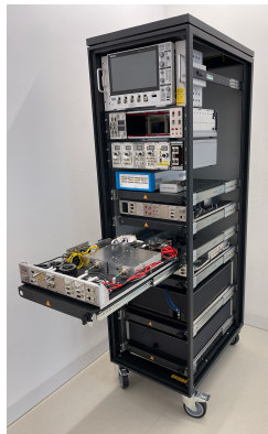
Figure 1. Stand-alone warm vapour QM system integrated in a 19” Rack, including the laser package and control electronics.
