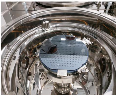
**Figure 1.** Picture of a wafer produced in one of the first batches placed inside the wafer bonder. Reservoir cavities and optical cavities that are patterned into the silicon preform are visible on the wafer surface.
