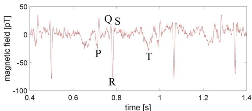
**Figure 1.** Real-time measurement of the magnetic field from a beating animal heart.
