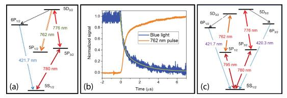
Figure 1. (a) Relevant energy levels of Rb atoms. (b) Directional blue light switching by the laser pulse at 762 nm. (c) Scheme of simultaneous excitation to the  $5D_{3/2}$  and  $5D_{5/2}$  levels.
